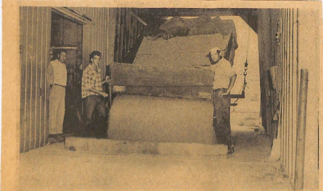
HANDLE WHEAT CROP — An important crop handled by the Oldcastle Co-op is wheat. During the three-week wheat harvest period the farmers line up with their wagons and the co-op has storage facilities to handle 60,000 bushels in a 24 hour period. Here, an electric hoist is dumping the wheat from a wagon into the grain cleaner.
